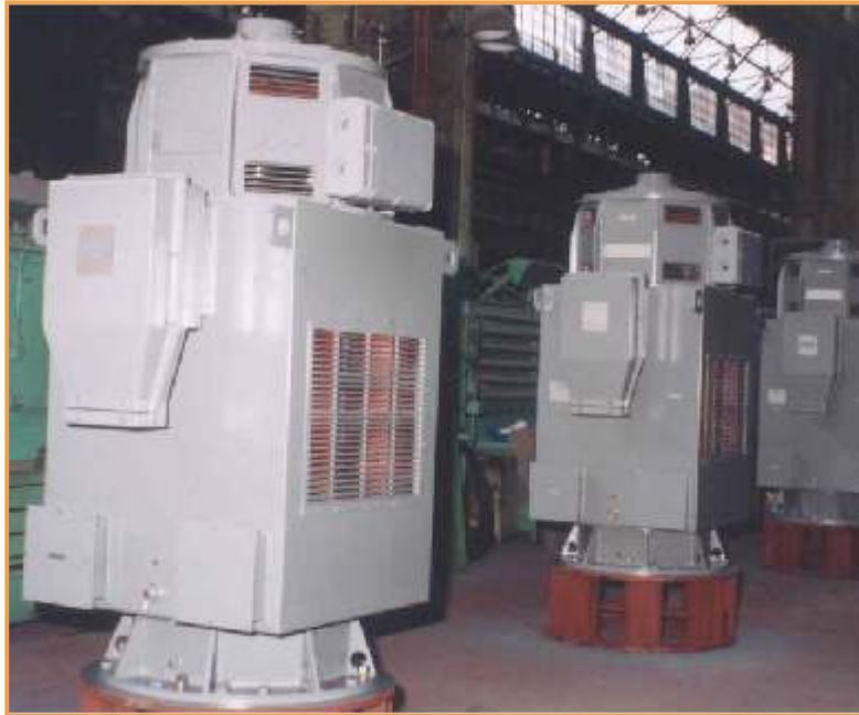
FHAV 450K6 type motor, 560 kW, 6.6 kV, 988 rpm.
