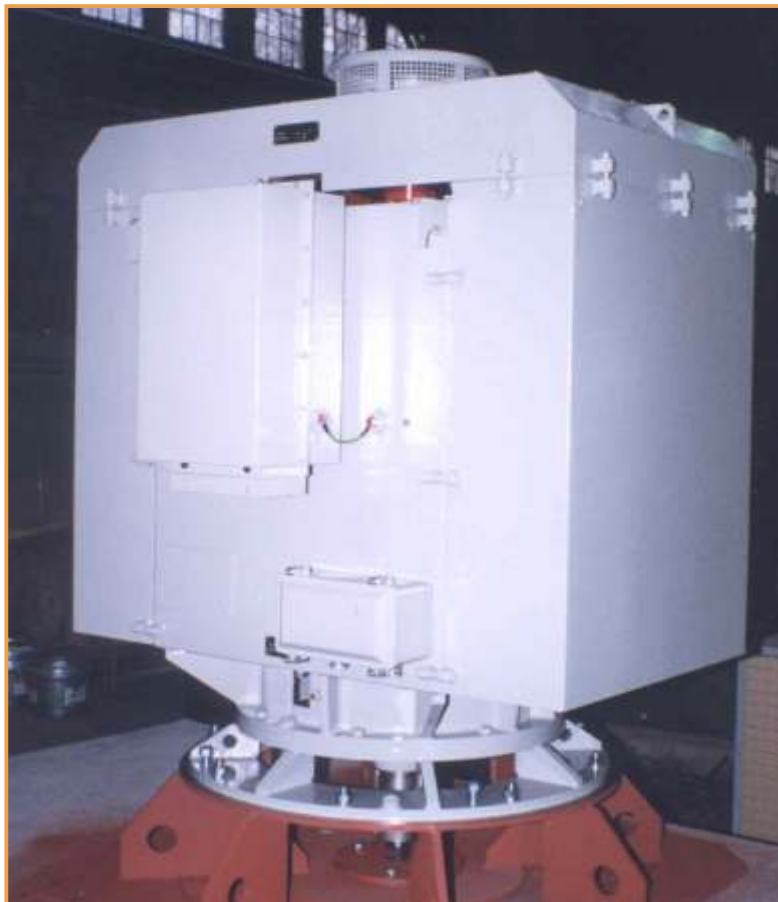
FTCV 400J6 type motor, 434 kW, 6 kV, 992 rpm.
